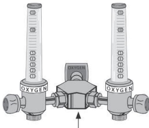
Flow splitting device (dual flow meter from a single wall source for use in two patients)
