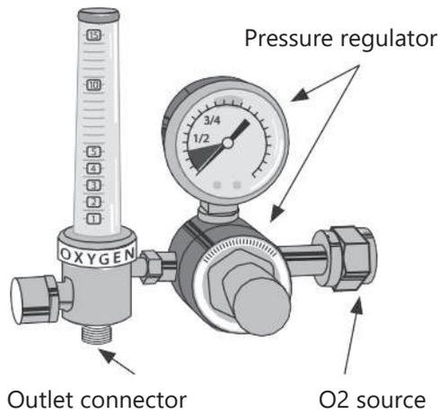
Thorpe Tube flow meter with pressure regulator and outlet connector
