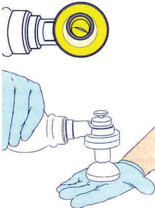
1. Squeeze the bag and check outlet valve whether opens or not
